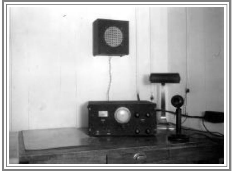
"Radio telephone receiver at Station KNDO which operates on 2496 K.C. Transcanyon communication with the North Rim summer headquarters supplement the telephone line during fire periods or other emergencies."
