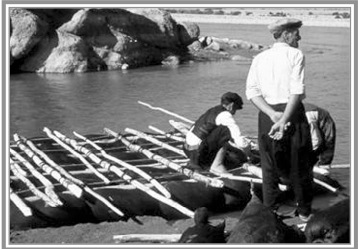
Frame pieces are attached to the inflated sheepskins which have been tied together to form rows of tubes.
